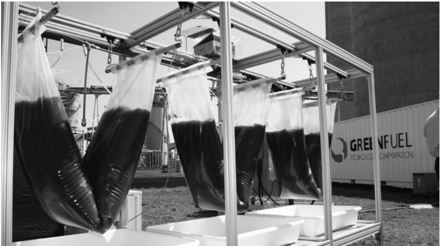
Figure 3-10. Operating Demonstration Algae Bioreactor at a Coal-Fired Power Plant in Louisiana.
