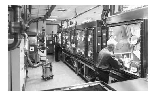
Figure 10 Glovebox line at the former Sellafield MOX Fuel Fabrication Plant. Source: UK Nuclear Decommissioning Authority.
