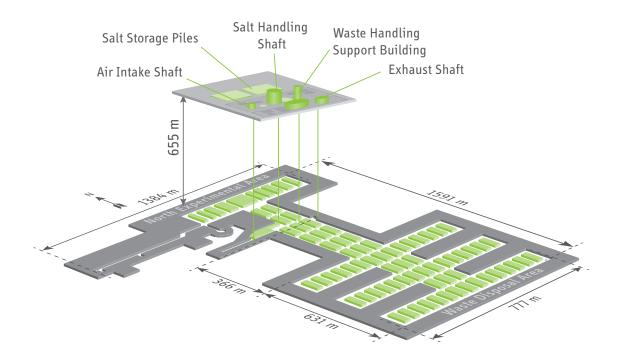
**Figure 9** The U.S. Department of Energy's Waste Isolation Pilot Plant (WIPP) near Carlsbad, New Mexico where plutonium-contaminated waste from weapons R&D and production is being disposed. *Source: Improving Operations and Long-Term Safety of the Waste Isolation Pilot Plant* (National Academy Press, 2001), Figure 1.2.
